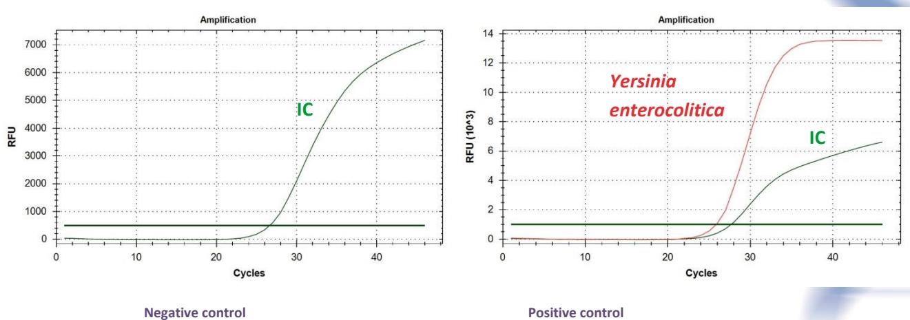
The result is considered invalid if there is signal of amplification in negative control or absence of signal in the positive well. We recommend to repeat the assay again.
